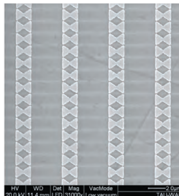
Nano-antenna array as produced in the Tel Aviv University Center for Nanoscience and Nanotechnology.
