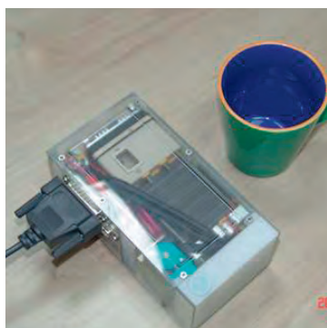
Fuel cell developed in Prof. Emanuel Peled's lab, operated by methanol and capable of powering a small laptop computer.
