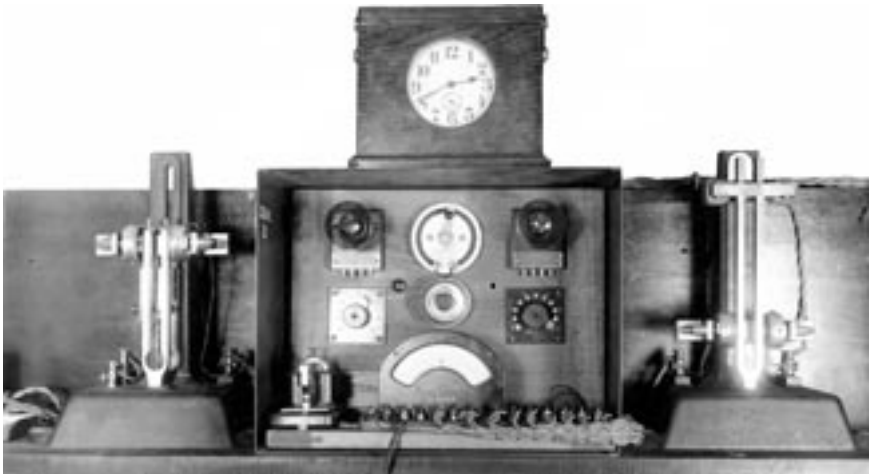
Figure 2. A clock connected to two tuning-forks at Western Electric research department, caption says from 14 November 1921. Notice that the clock is connected (probably alternatively) to two forks of different dimensions. The left one is excited by magnets near its upper part and the right one by magnets near its lower part. (Courtesy of AT&T Archives and History Center)
